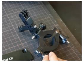
Put the two spacers into the two gaps of the extension piece's top respectively. Use a tool to adjust the hole and adjust accordinly so the circluar parts are aligned for the long screw to go through.
