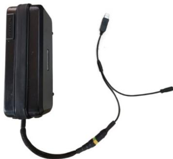
Plug the USB to the PC's USB port. The opposite end of the programming cable is connected to the main connector of the wiring harness. Afterwards, connect the DS103 display to the display connector of the wiring harness.
