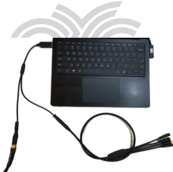
Plug the USB to the PC's USB port. The opposite end of the programming cable is connected to the main connector of the wiring harness.
