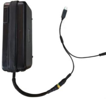
Connect the programming cable to the battery, then plug the USB to the PC's USB port.
