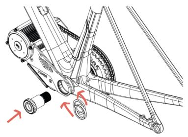
3. Insert the spindle from the right (drive) side. Note that you will need to line up the splines from the chainring assembly. If your spindle does not go through or comes to a hard stop before being fully inserted, rotate the spindle slightly and try again. Once the spindle is lined up, a soft tip hammer may also be used to get the spindle all the way through. Add a little grease on the o-rings and the torque sensor splines.
