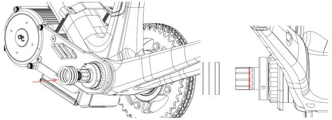
on your crank arms. Use the M15 ISIS crank arm screws to tighten and secure the crank arms.
