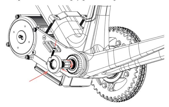
5. Install the motor hanger (see page 29) and place the rubber padding provided in between the motor and the frame.
