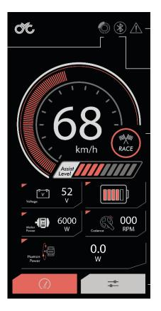
Warning icon to check error codes & clear faults
