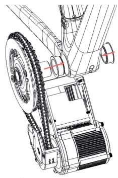
2. Line up the motor body with your frame at the bottom bracket and insert the right (drive) side of the motor into the frame's bottom bracket shell.
