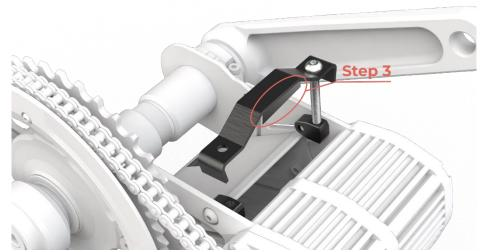
4. Place the second aluminium joint on the other side of the mounting bracket & connect the hanger fully. Tighten the hanger to ensure that the motor is secured.
