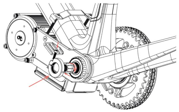
5. Install the motor hanger (see page 32) and place the rubber padding provided in between the motor and the frame.
