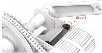
1. Place one of the aluminium joints on the inside of the bracket & screw in the bolt to attach it to the motor's mounting plate.
