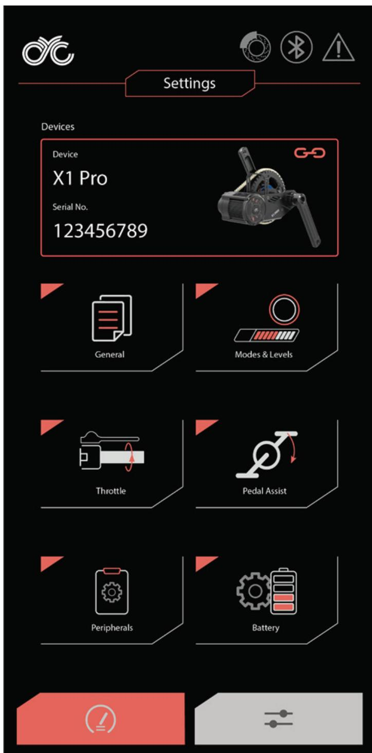
The settings page allows you to navigate through different parameter categories. There are six different categories with each providing a set of adjustable parameters or readings from your ebike system.
